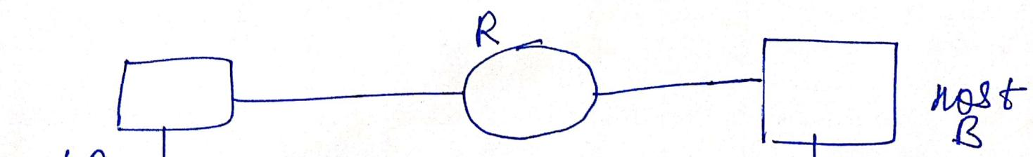
if the router will not found the route packet then router discard the ~~msg~~ packet
