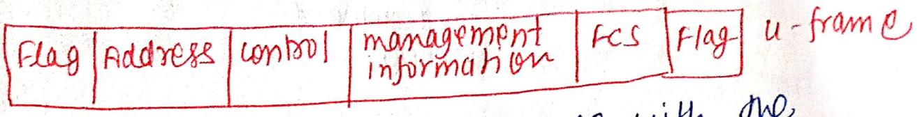
Flag field - it is a 8 bit sequence with the bit pattern 01111110 that identifies both the beginning and end of the frame
